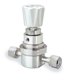
TESCOM 74-3800 Series ultra high purity, tied diaphragm pressure reducing regulator offers high flow and internally threadless and low internal volume design with  $C_V = 0.5$ . The 74-3800 Series is available with 10  $R_a$  surface finish. Inlet pressures are 600, 1000, or 3500 psig / 41.3, 69, 241 bar with outlet pressures up to 150 psig / 10.3 bar.
