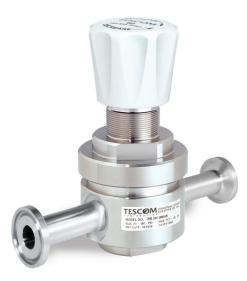
TESCOM PH-3200 Series is part of our Pharmpure<sup>™</sup> product line. This high purity high flow singlestage regulator offers a compact, USP Class VI and BPE compliant design suitable for biotech and pharmaceutical applications. This regulator offers gas flows of 5-50 SCFM / 142-1416 SLPM. Diffusionresistant metal-to-metal diaphragm seal ensures gas purity and integrity.
